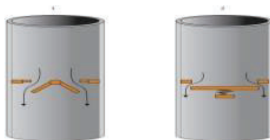
FIGURE 30: SCHEMATIC REPRESENTATION OF NON-RETURN VALVE (LEFT) CLAPPER TYPE AND (RIGHT) SPRING TYPE
