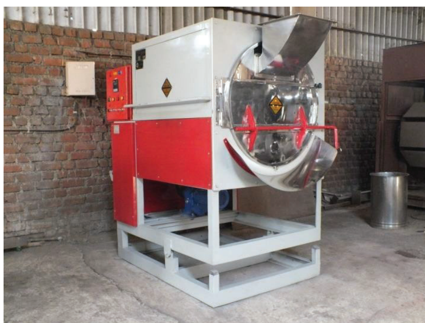
FIGURE 26: PICTURE OF ROTARY DRYER (FOR REPRESENTATION PURPOSE ONLY; NOT TO THE SCALE)
