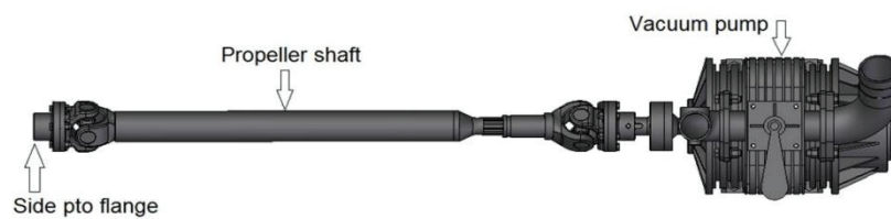
FIGURE 31: SCHEMATIC REPRESENTATION OF VACUUM TRUCK WITH 4 CUM CAPACITY AND ITS VACUUM SYSTEM AND DRIVE SYSTEM
