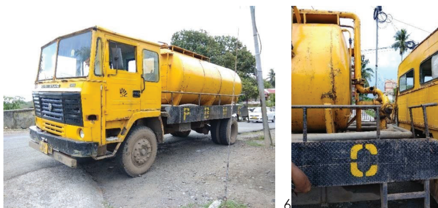
FIGURE 8: VACUUM TRUCK OF 8 M 3 CAPACITY MANAGED BY PBMC
